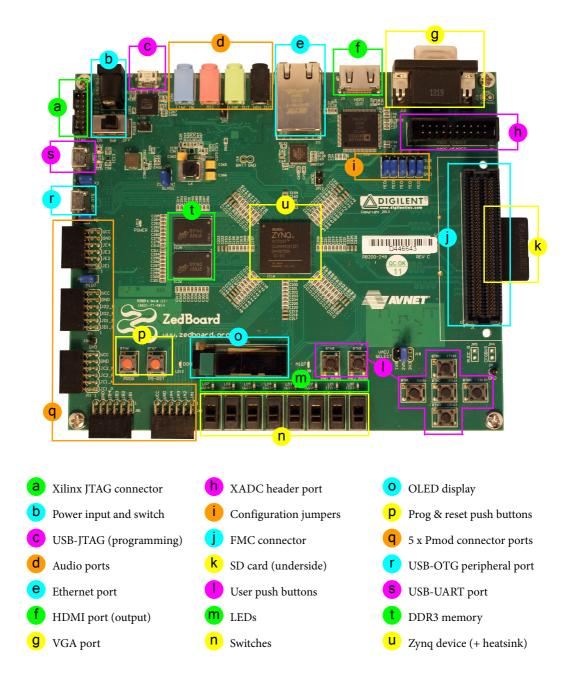
Figure 6.1: ZedBoard layout and interfaces (front)
