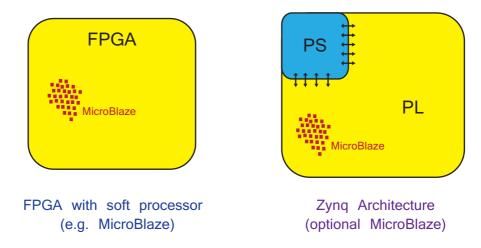
*Figure 4.2: Comparison between an FPGA with soft processor (MicroBlaze), and a Zynq device with hard processor (ARM) and optional soft processor (MicroBlaze).*
