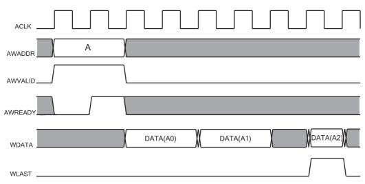
Figure 19.3: Simplified AXI4 write burst transaction
