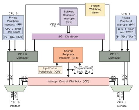
Figure 10.7: Interrupt controller block diagram
