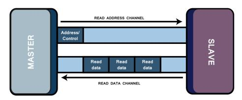
Figure 19.2: AXI4 read channel architecture
