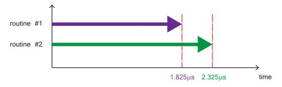
Figure 4.4: Visualisation of processing time for two variations of a software routine
