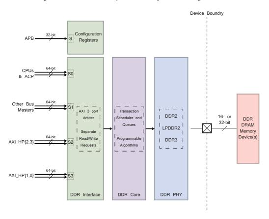
A block diagram of the DDR memory controller is provided in Figure 10.3.
