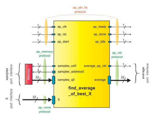
*Figure 15.11: RTL interface diagram for the 'find\_average\_of\_best\_X()' function, showing both default port level ports and protocols, and default block level ports and protocol*
