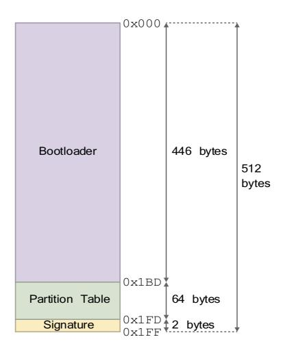
Figure 24.2: Structure of the Master Boot Record (MBR)
