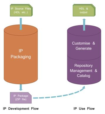
Figure 18.3: IP packaging and use flow
