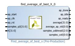
*Figure 15.12: An IP Integrator block produced for the "find\_average\_of\_best\_X" function, with port- and block-level protocols as specified in Figure 15.11.*
