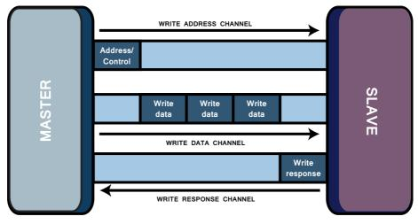
Figure 19.1: AXI4 write channel architecture
