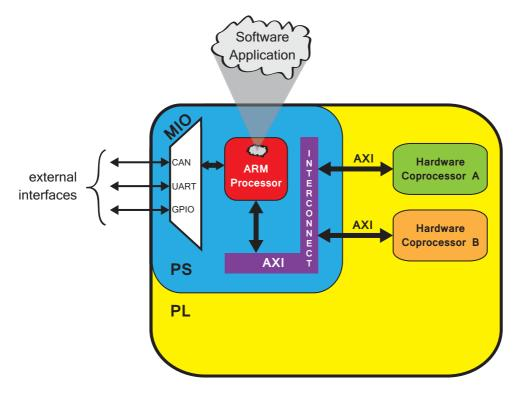
Figure 3.3: Conceptual diagram of an example hardware system with MIO
