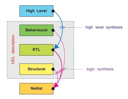
Figure 14.2: High level synthesis and logic synthesis
