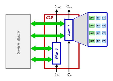
Figure 2.6: Composition of a Configurable Logic Block (CLB)
