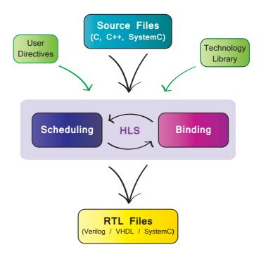
Figure 14.7: Vivado HLS scheduling and binding processes
