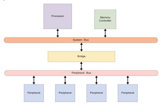
Figure 9.2: Generic embedded system architecture
