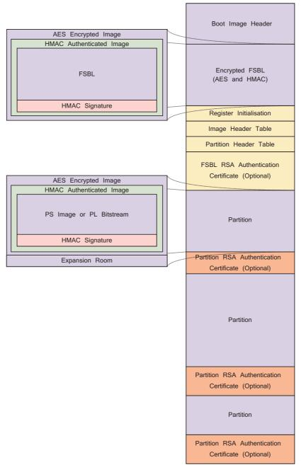
Figure 24.7: Zynq Boot Image Format (BIF) structure
