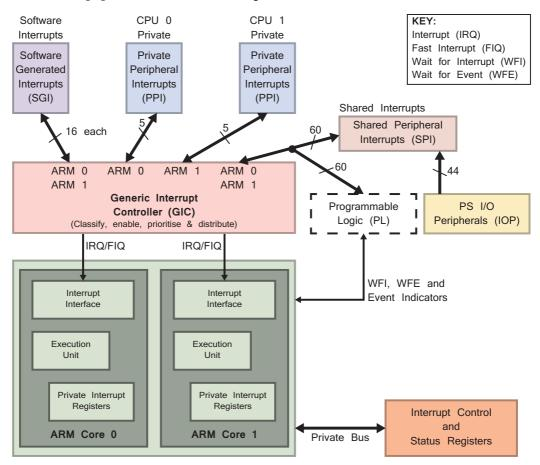
Figure 10.6: System-level interrupt environment
