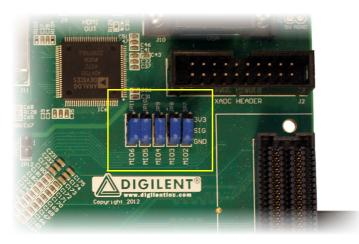
Figure 6.4: The set of jumpers determining configuration options
