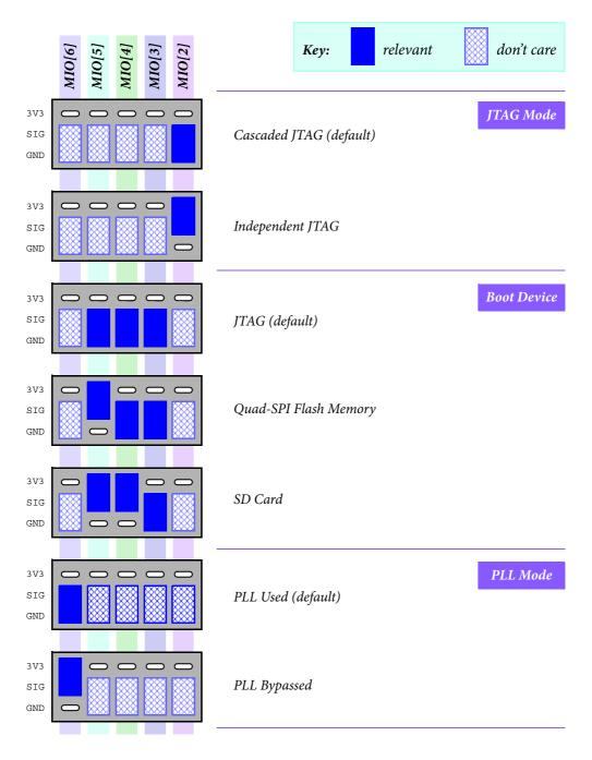
Figure 6.5: Jumper settings for all ZedBoard configuration options
