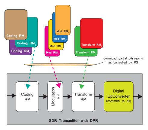
Figure 5.10: A flexible SDR architecture using DPR
