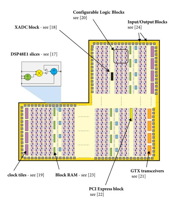
Figure 2.13: Programmable Logic - references
