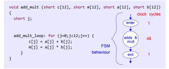
Figure 15.25: Merged addition and multiplication loops
