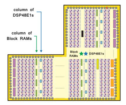
Figure 2.7: The logic fabric and its constituent elements
