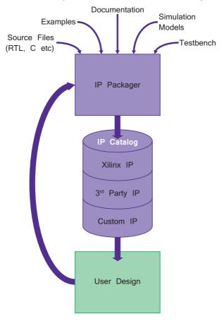
Figure 18.1: Vivado IP-centric flow
