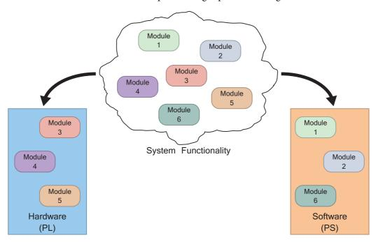
An overview of hardware/software partitioning is provided in Figure 11.1.
