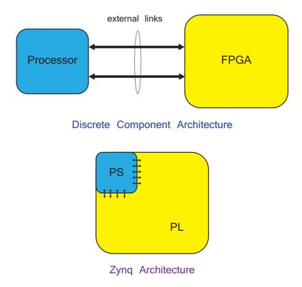
*Figure 4.9: Comparison between discrete-component and Zynq-based combinations of processing system and programmable logic*
