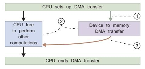
Figure 9.8: DMA memory transfer operation
