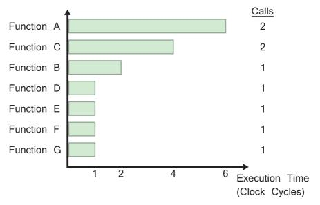
Figure 11.4: Example profiling results with reference to Figure 11.3
