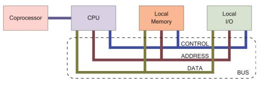
Figure 9.7: Bus comprised of control, address and data lines
