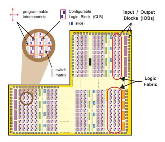
Figure 2.5: The logic fabric and its constituent elements
