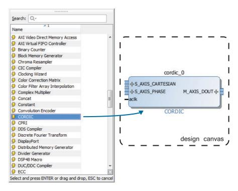
Figure 3.6: A CORDIC IP block is introduced into an IP Integrator system from the catalogue
