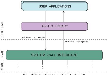
Figure 23.2: Simplified interrupt based system call
