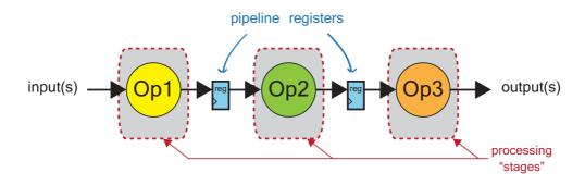
Figure 15.18: Partitioning of operations into separate stages via pipelining
