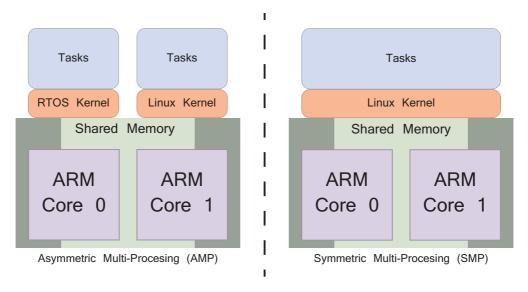
Figure 21.3: Asymmetric vs. symmetric multi-processing
