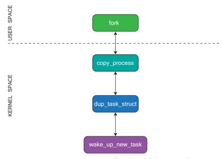
Figure 23.4: Process creation flow through fork system call
