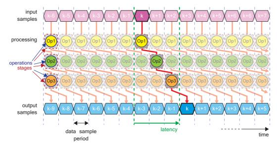
Figure 15.19: Waveform showing throughput and latency, after pipelining
