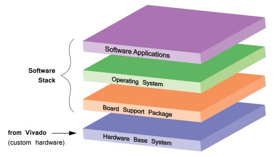
Figure 3.5: Hardware and software layers of a Zynq design
