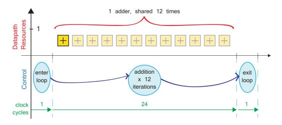
Figure 15.23: Extraction of addition loop into datapath and control logic
