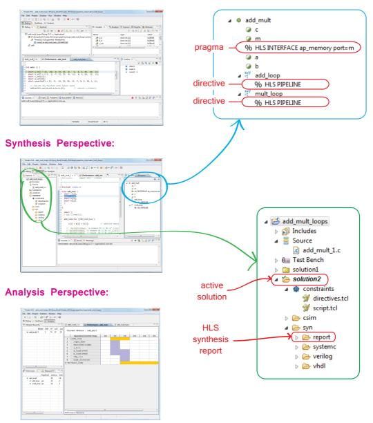
Figure 15.2: Overview of Vivado HLS GUI perspectives
