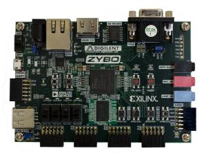
Figure 3.9: The ZYBO Development Board
