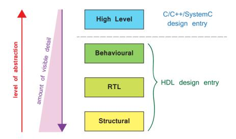
Figure 14.1: Levels of abstraction in FPGA designs
