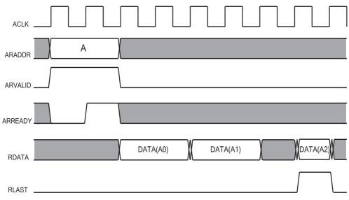
Figure 19.4: Simplified AXI4 read burst transaction
