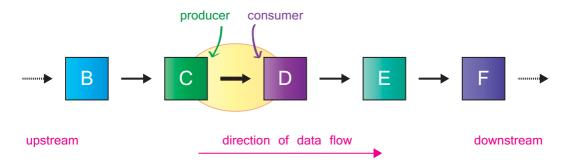
Figure 15.10: Data flow between Vivado HLS blocks
