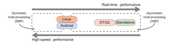
Figure 21.2: Embedded operating system performance
