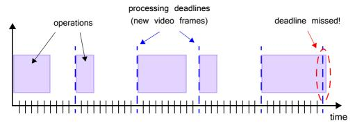
Figure 4.6: Real-time processing
