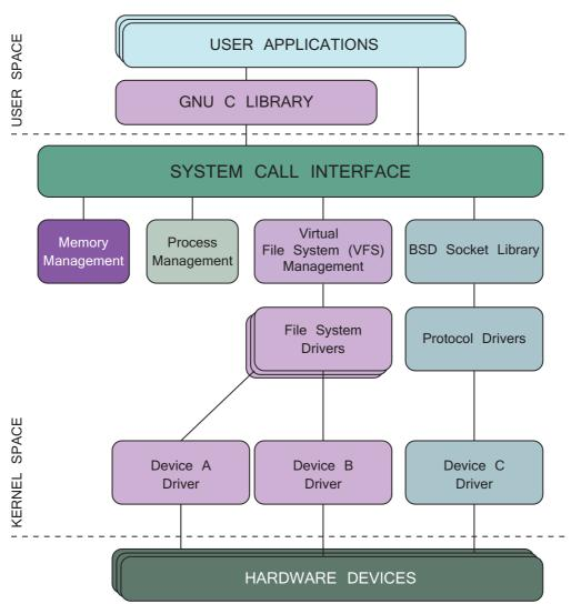
Figure 23.1: Important components of the Linux kernel
