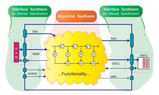
Figure 14.4: Clarification of the algorithm and interface, and showing a subset of interface types
