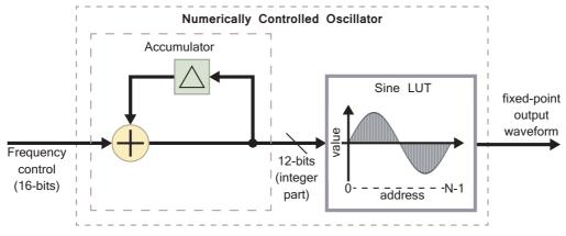
Figure 17.2: Architecture of a Numerically Controller Oscillator (NCO)
