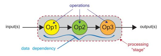
Figure 15.16: Example function with data dependencies between operations
