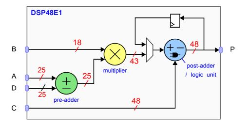
Figure 2.8: Arithmetic capabilities of the DSP48E1 slice
