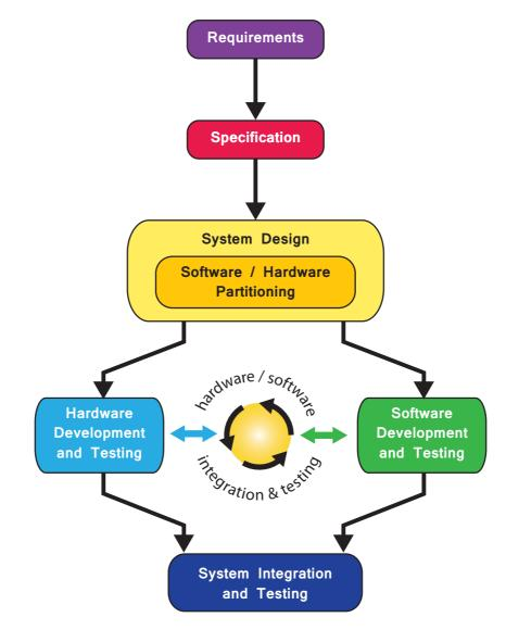
Figure 1.5: A basic model of the design flow for Zynq SoC
