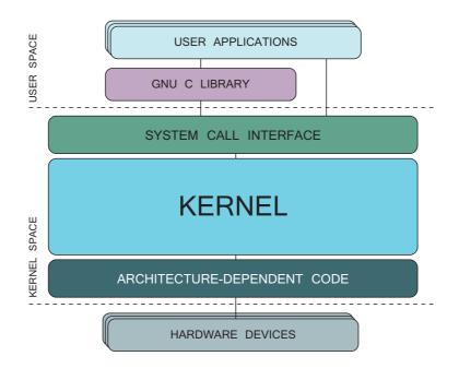
Figure 22.1: A High-level GNU/Linux system architecture
