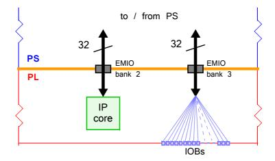
Figure 2.10: Using the EMIO to interface between PS and PL
