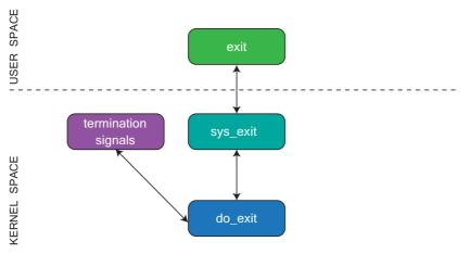
Figure 23.5: Operation of process destruction
