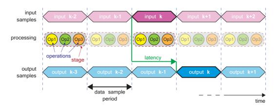
Figure 15.17: Waveform showing throughput and latency, before pipelining
