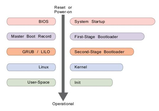
Figure 24.1: Stages of the desktop Linux boot process
