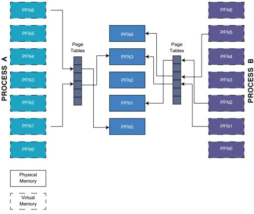
Figure 23.3: Simplfied representation of virtual memory[2]
