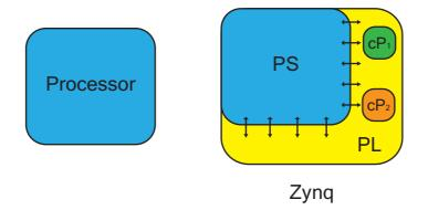
*Figure 4.8: Comparison between a processor alone, and a small Zynq device*
