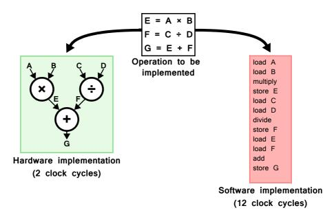
Figure 11.2: Parallel vs sequential implementation
