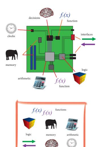
Figure 1.1: Comparison of System-on-a-Board (top) and System-on-Chip (bottom)
