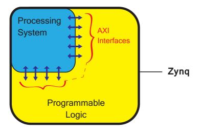
Figure 1.2: A simplified model of the Zynq architecture
