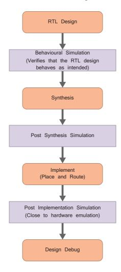
Figure 13.5: Vivado RTL simulation flow
