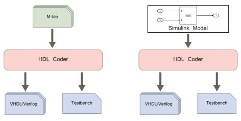
Figure 13.3: HDL Coder flow
