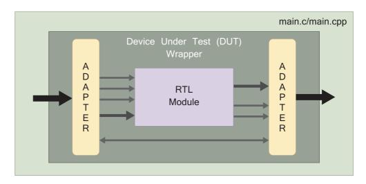
Figure 13.6: RTL co-simulation wrapper
