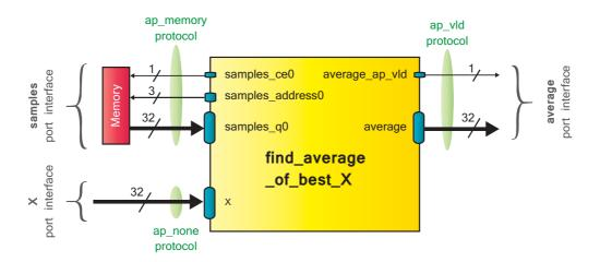
*Figure 15.9: RTL interface diagram for the 'find\_average\_of\_best\_X()' function, showing default port level ports and protocols*
