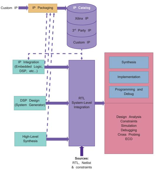
Figure 18.2: Vivado Design Suite system-level design flow
