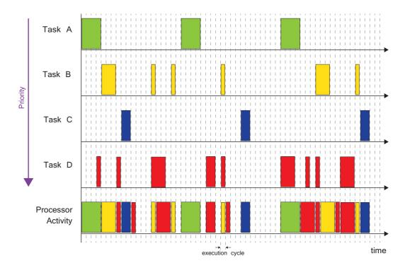
Figure 4.5: Processor operation: execution cycles
