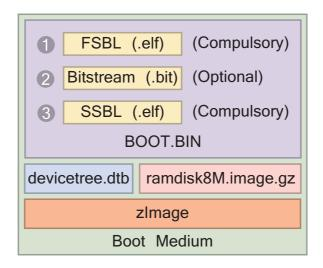
Figure 24.5: Required files for Zynq Linux boot medium
