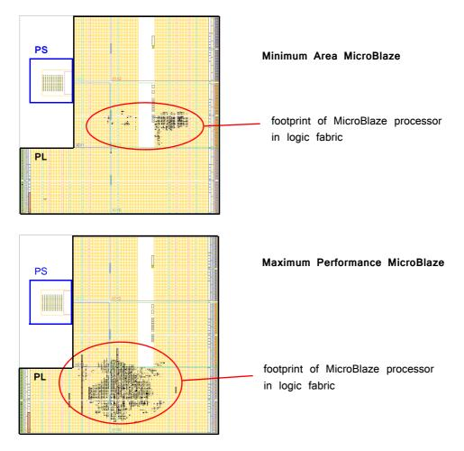
*Figure 4.1: Floorplans of 'minimum area' (top) and 'maximum performance' (bottom) MicroBlaze soft processor implementations*
