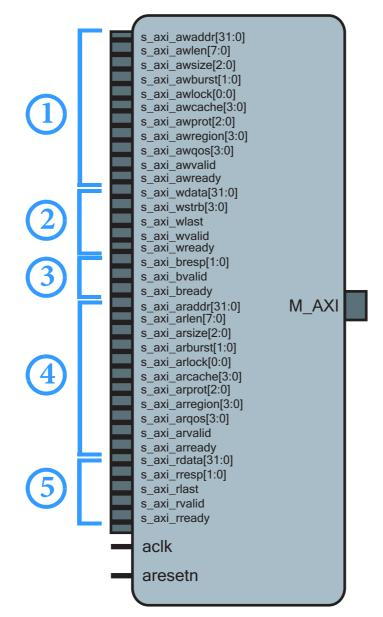
Figure 19.6: Representative AXI4 data FIFO in Vivado IP Integrator (bus expanded)
