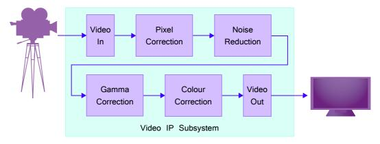
Figure 13.1: Video IP subsystem
