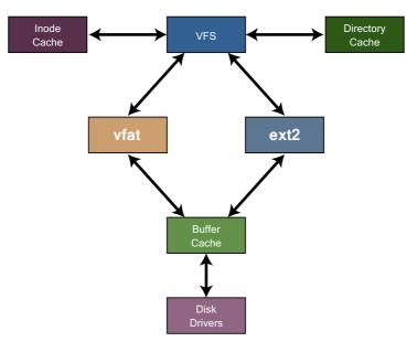
Figure 23.6: Linux virtual file system interactions[5]
