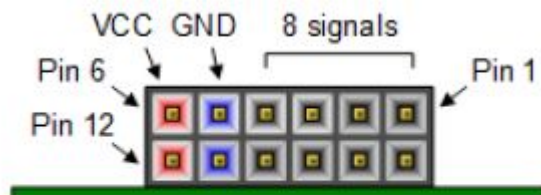
Figure 20. PMOD connectors; front view, as loaded on PCB.
